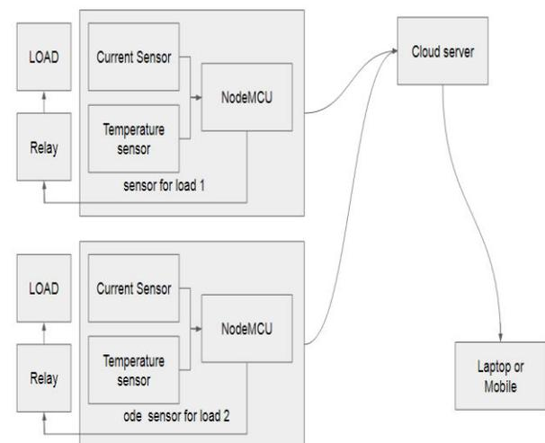
**Figure 1 Block Diagram of the Proposed System**
